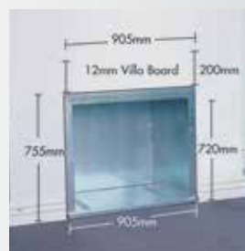
Zero Clearance Box positioned in framework mounted on 12mm Villa Board cut out size. (Box size: 905w x 720h) (Cut out size: 905w x 755h)
