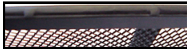
Mesh fitted between main frame and welded back strip
